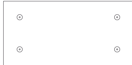
4 fixings per board Recommended fixing pattern for 4 fixing per board (1200mm x 600mm board - 5.56 fixings/m 2 )
