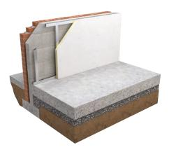
**6.** Seal and tape the joints of the plasterboard to ensure a continuous vapour control layer is created Fill any gaps with foam filler or equivalent.
