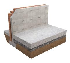
3. Fix the metal frame system/vertical timber battens at a maximum of 600mm centres (incorporating a vertical DPC behind timber battens). Ensure framing system/battens are wide enough to offer 20mm support to all four edges of the plasterboard. Pack battens, if necessary, to level the wall. Extra noggins may be required when the XT/TL-MF is unsupported by the battens/studs.
