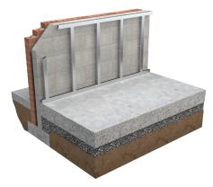
4. Lift the insulation board into position using wedges on the floor. Insulation should be cut back to accommodate an adjoining panel at external corners. Joints should be tightly butted. 5. Fix the Thermal Liner to the frame at 300mm centres using appropriate fixings e.g. drywall screws, at least 12mm in from the board edge. The fixings should penetrate at least 25mm into the battens/ studs. Fixings should be thermally broken where possible. For specific guidance contact fixing manufacturer.
