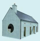
Y = 0.08 (Acceptable Details) The equivalent of an open 'Patio Door' 2.1m x 1.8m (3.78m<sup>2</sup>) opening.
