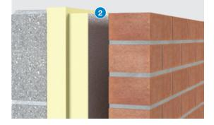
**3.** The textured robust low emissivity foil facing on XtroWall Plus improves the thermal performance of the wall. The residual cavity is the most effective method of preventing wind-driven rain penetrating a wall from the outside.
