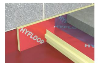
4. Good detailing at the wall/floor junction is essential to reduce Thermal Bridging. By placing an upstand of Unilin Perimeter strip insulation with a minimum 25mm thickness around the external and internal wall/floor junctions, a robust detail is created.
