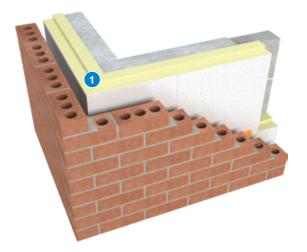
2. The XtroWall Plus engineered jointing offers a practical on-site solution that results in a more robust continuous layer of insulation, minimising the threat of Thermal Bridging and improving the overall U-Value of the wall.
