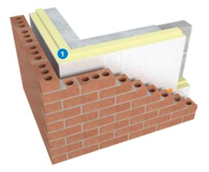
2. The XtroWall engineered jointing offers a practical on-site solution that results in a more robust continuous layer of insulation, minimising the threat of Thermal Bridging and improving the overall U-Value of the wall.
