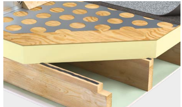
Typical Installation - Timber Deck
